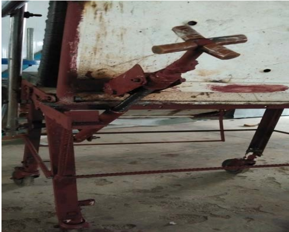
Fig. 3 Lead Screw Mechanism
